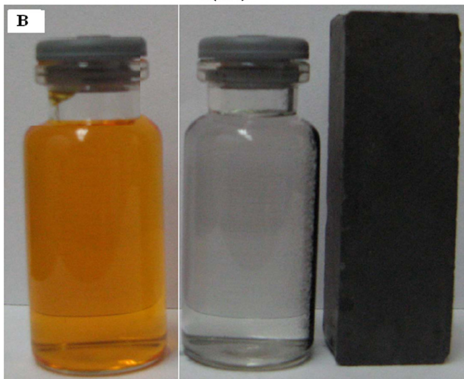
Fig. 6. The magnetization curves (A) for the Ni-OMCs and images of the magnetic separability (B).
